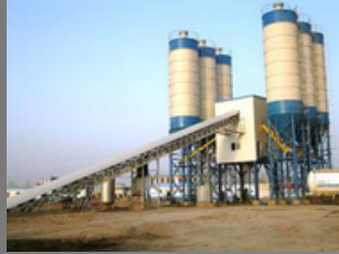
Batching Plant 1 Nos. 30 M 3
